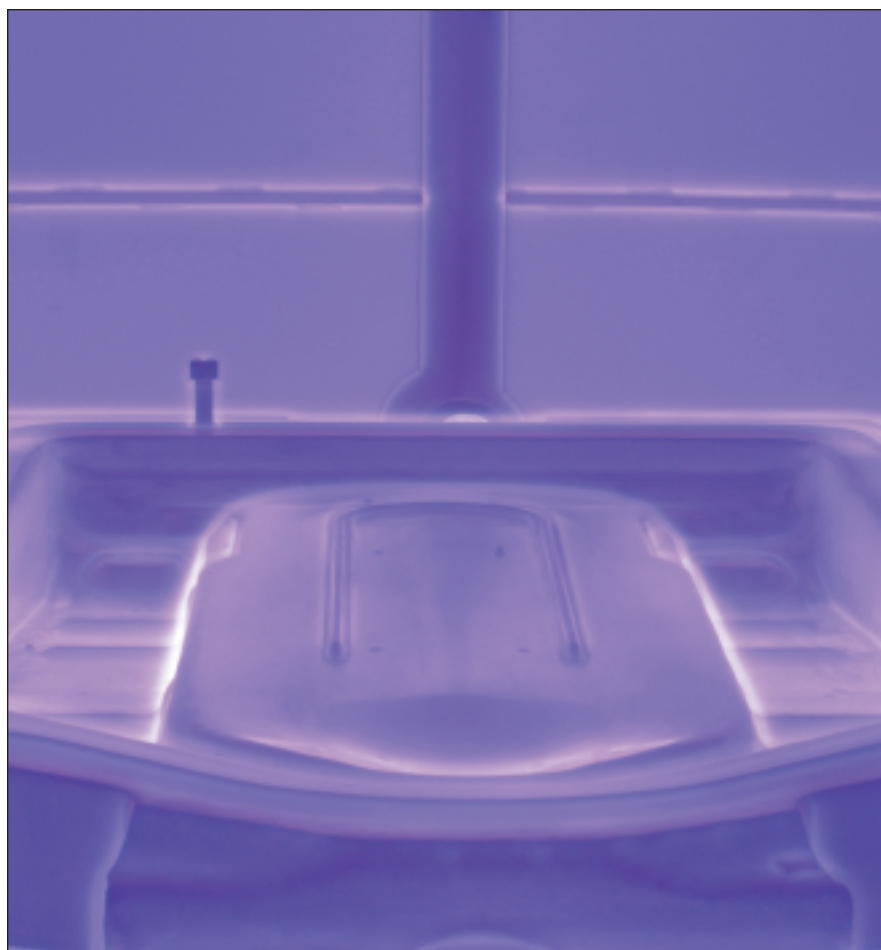
View of a large stamping die undergoing plasma nitriding in a vacuum chamber.
