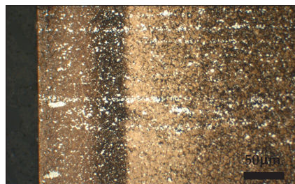
Fig. 4 — Hardness profile in the M2 sample plasma nitrided at 900°F; total case depth is 0.0036 in.
