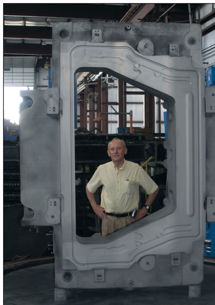
Fig. 1 — Examples of large automotive stamping dies after plasma nitriding at Advanced Heat Treat Corp. Monroe, Mich., facility.
